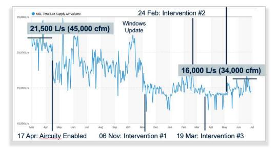
The key point demonstrated in this example is that UBC was able to track the results of interventions and adjustments to the new system easily in SkySpark and achieve the performance expected with the investment in the airflow management system.
