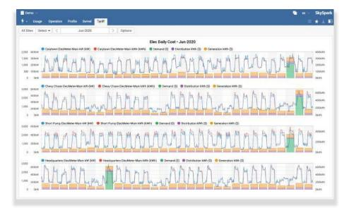
In this view, the lines represent consumption (kWh) and demand (kW) and the vertical bars represent energy cost calculated based on actual tariff rate charges.
