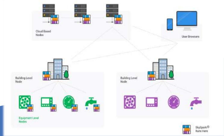
**Distributed Architecture** – By this we mean that SkySpark can be deployed on multiple nodes (computing devices) distributing the work of data collection, analytics processing and presentation of results to users.
