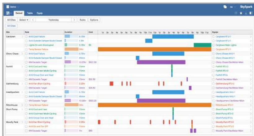
FDD is one subset of the overall capabilities provided by data analytics. This image shows fault patterns as timelines
