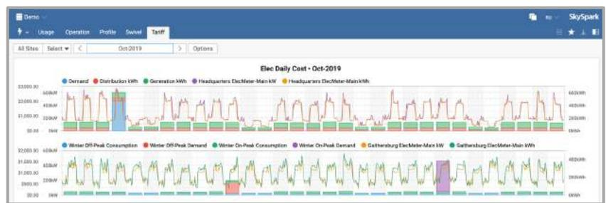
Image showing correlation of energy consumption and demand (line charts) with tariff-based cost calculations (bar charts)
