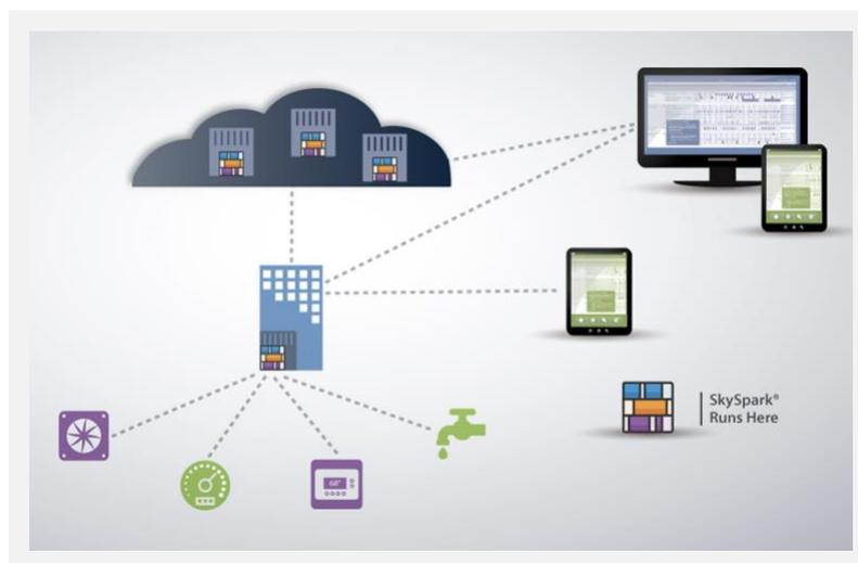
In this architecture, a node running SkySpark is installed in the facility and connected to local data sources via a variety of standard data acquisition connectors including: Bacnet® IP, Modbus TCP, Obix™, Haystack, SNMP, Sedona, OPC UA, SQL, and the REST API – all included with SkySpark as a standard feature.
