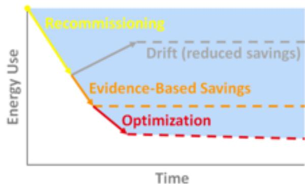
Figure 1. Energy savings can diminish over time. ETC Group uses real-time monitoring to maximize initial savings and uncover additional optimization opportunities over time
