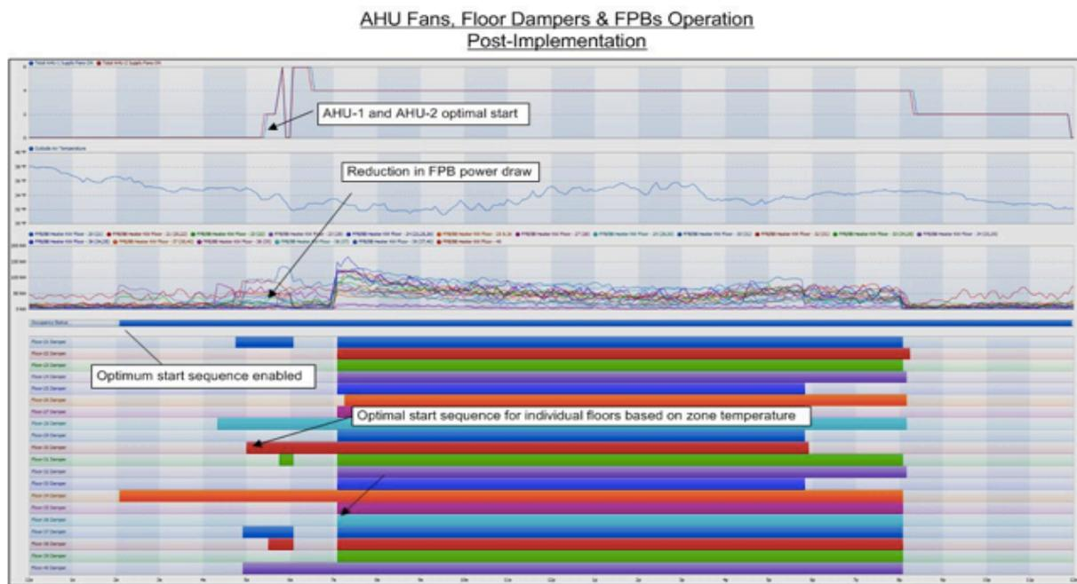
Graphic shows operation of AHU fans, floor dampers, and FPB operation after implementation of a staged optimum-start control sequence
