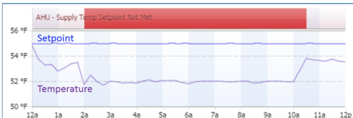
Figure 2. Automatic Fault Detection (in red above) reveals when a piece of equipment cannot meet its temperature setpoint. This fault indicates the potential to save energy by reducing unnecessary cooling.
