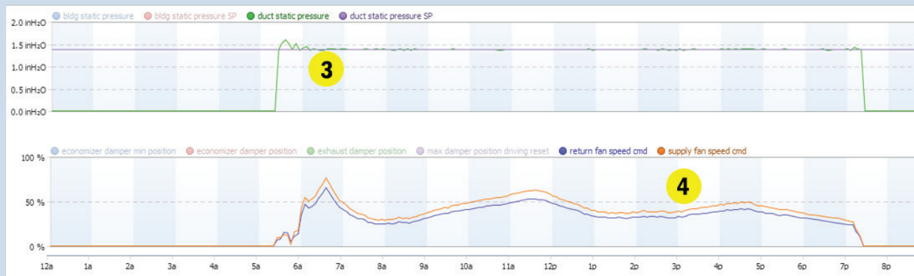
Figure C: Current Fan Speed and Static Pressure Control
