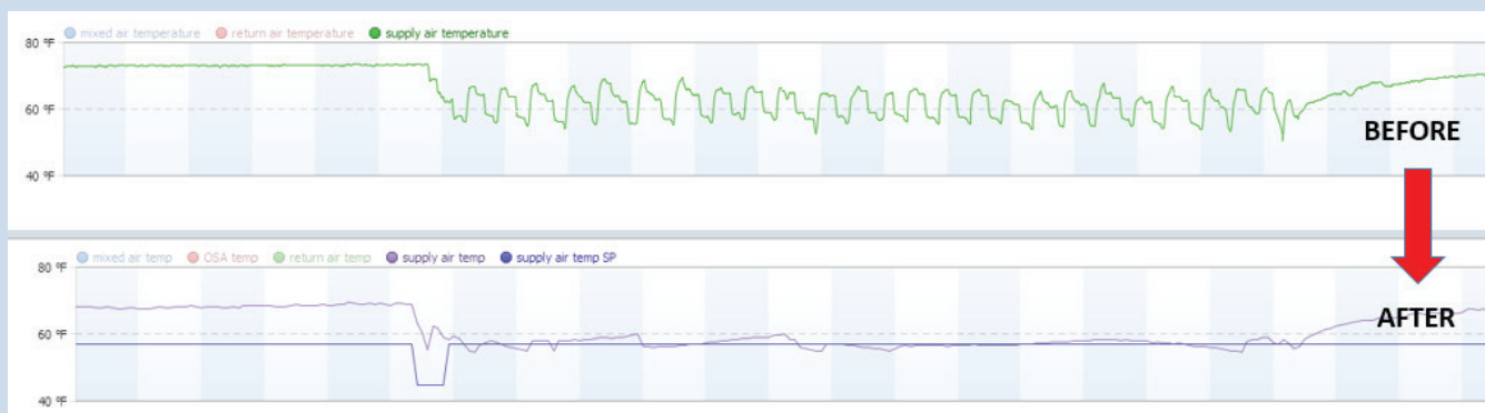
Figure A: Before and After Supply Air Temperature Control. Note the significant cycling of supply air temperature from the unit before the changes. As a result of the improvements, occupant comfort is greatly improved and the lifetime of compressors is extended.
